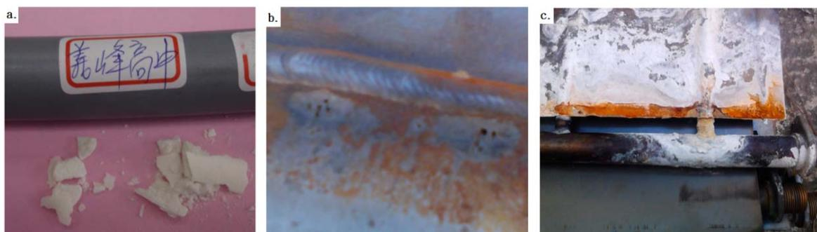
**Figure 2.** (a) Scaling in the connecting pipe; (b) pitting corrosion near the weld on storage tank; (c) corrosion and scaling on solar collector.
