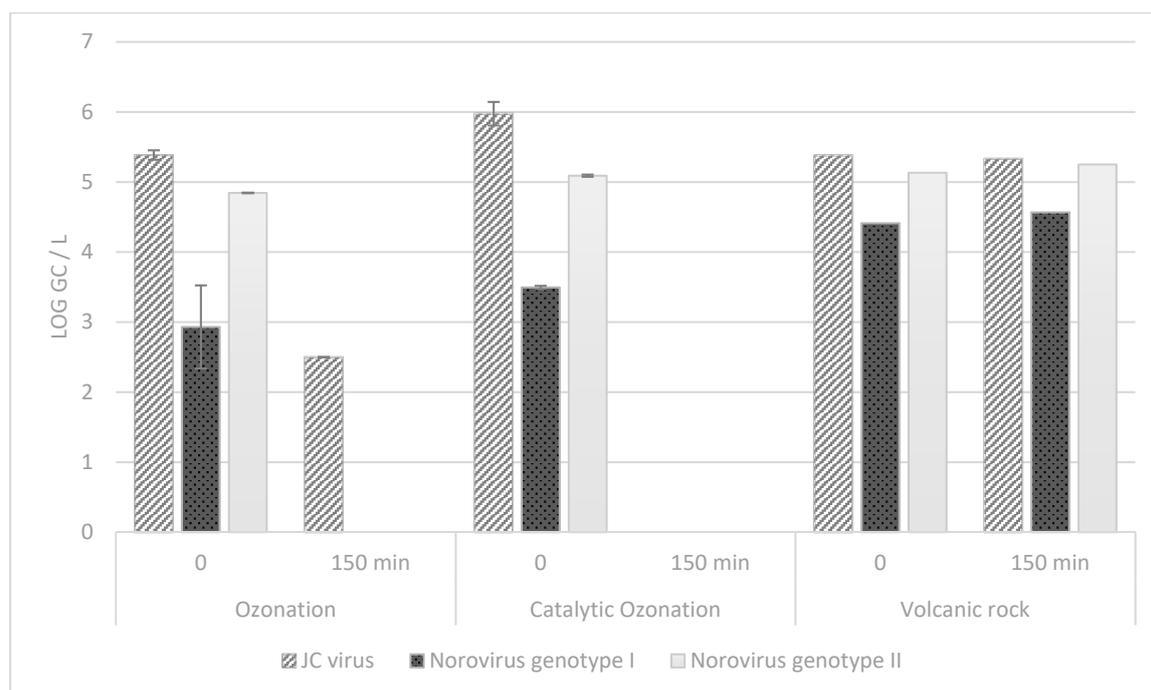
**Figure 3.** Initial and final virus concentration after single ozonation, catalytic ozonation, and contact with the catalyst.
