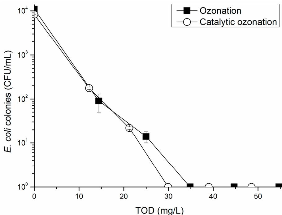
**Figure 1.** *E. coli* concentration using single and catalytic ozonation as function of TOD (using log<sub>10</sub>scale).
