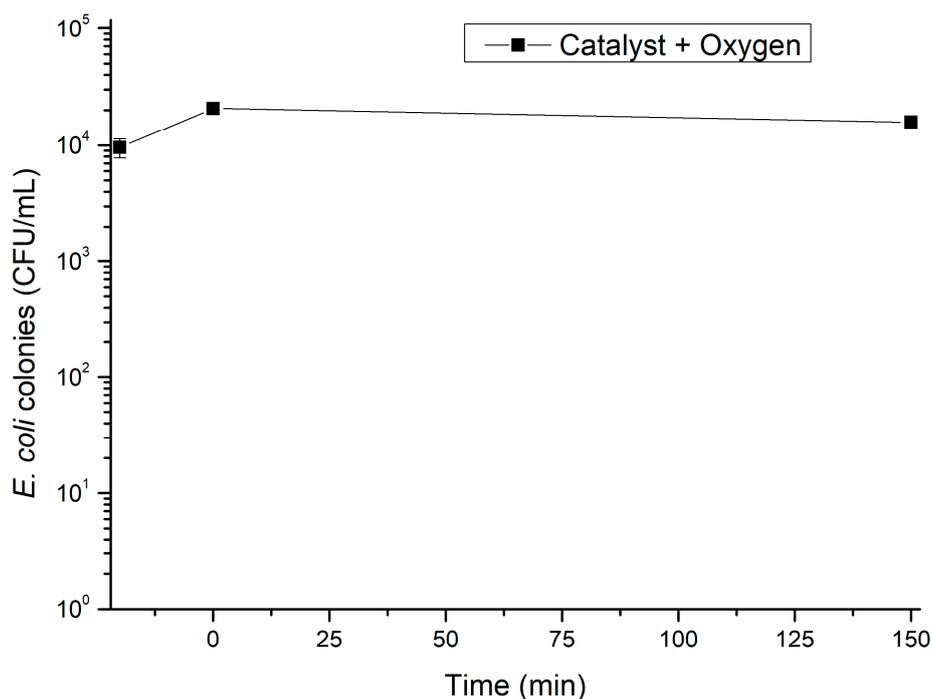
**Figure 2.** *E. coli* concentration using wastewater and volcanic rock as a function of time (−20 to 0 min without oxygen and from 0 min bubbling O<sub>2</sub>, using log<sub>10</sub> scale).
