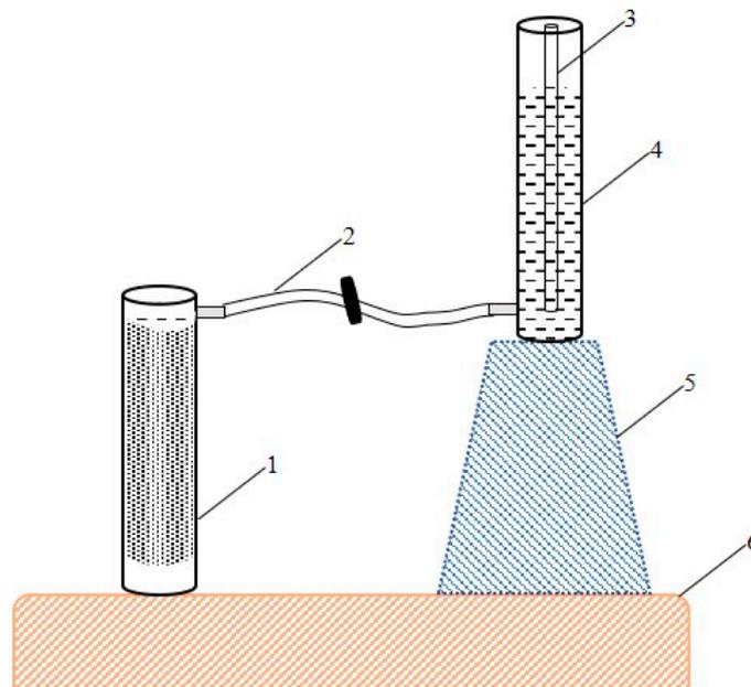
**Figure 1.** Experimental setup for one-dimension vertical water infiltration. (1) Soil column; (2) Water pipe; (3) Intake tube; (4) Markov bottle; (5) Retort stand; and (6) Desktop.
