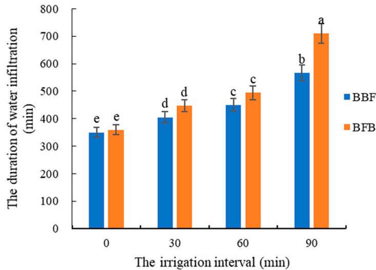
**Figure 3.** Effects of different irrigation treatments (BBF, brackish-brackish-fresh water; BFB, brackish-fresh-brackish water) on the duration of water infiltration in the silty loam. Different letters above columns indicate significant differences ( $P < 0.05$ ).
