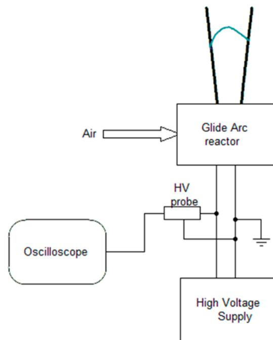
**Figure 1.** Scheme of the gliding arc plasma reactor.
