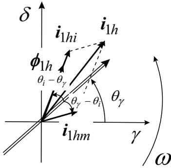
Fig. 7. Relation among phases of rotor-N-pole, in-phase current and mirror-phase current.
