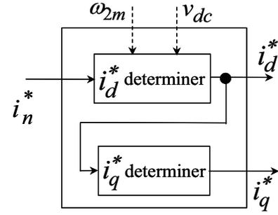
Fig.9. Basic configuration of the command converter
