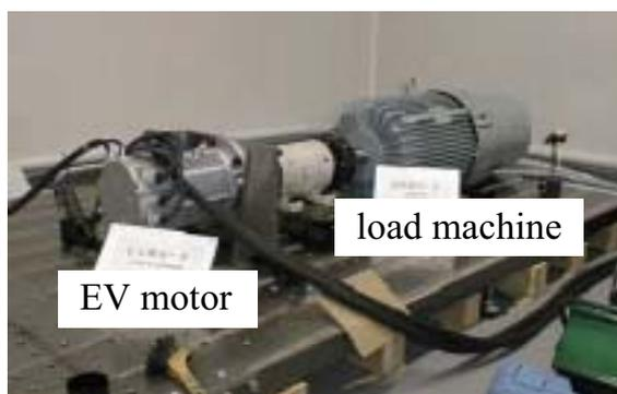
Fig. 13. SP-PMSM for ST-EV on test bed.
