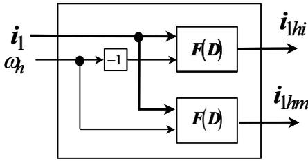
Fig. 8. Configuration of the in-phase mirror-phase current evolver based on filters in the D-module.
