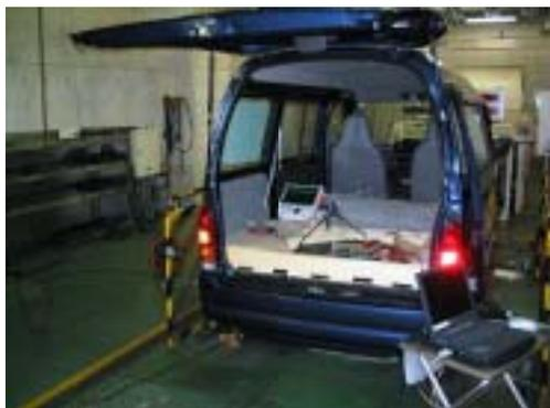
Fig. 17. ST-EV on chassis dynamometer.
