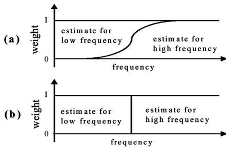
Fig.3. An example of frequency weight for frequency hybrid.
