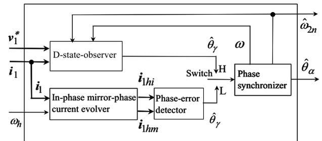
Fig. 4. Configuration of the phase estimator.
