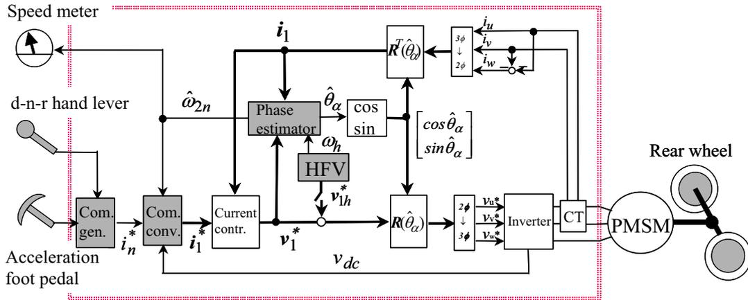
Fig. 2. Basic configuration of drive control system for ST-EVs.
