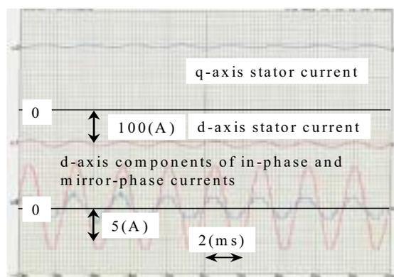
Fig. 15. A response of SP-PMSM producing rated 40-Nm torque at standstill.
