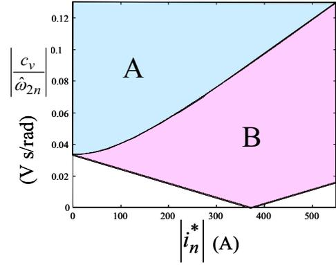
Fig. 10. Attainable operation region under voltage limit.
