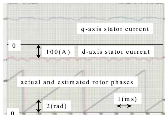
Fig. 14. A response of SP-PMSM producing rated 40-Nm torque at speed of 400-rad/s.
