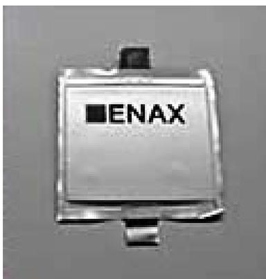
Fig. 6 Laminate sheet type lithium ion cell (Weight: 190g, D170mm x W160mm x H5mm)
