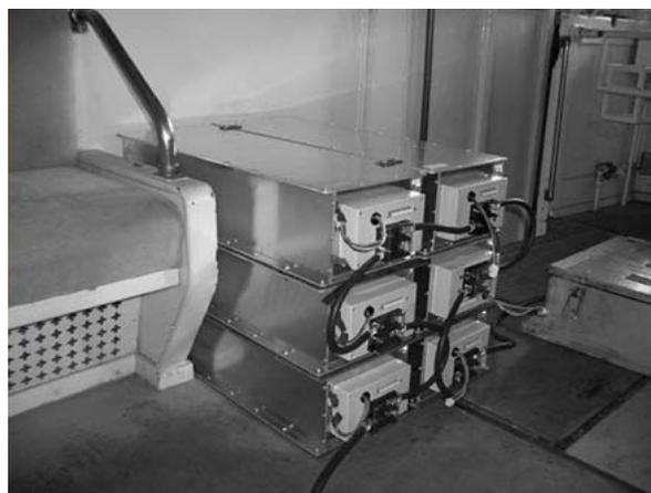
Fig. 8 20kWh type lithium ion battery module
