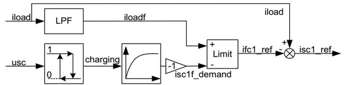
Fig. 9 Current reference of the supercapacitor [7]
