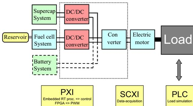
Fig. 10 Test setup of the series hybrid propulsion system using a fuel cell as energy source and a supercapacitor as peak power unit
