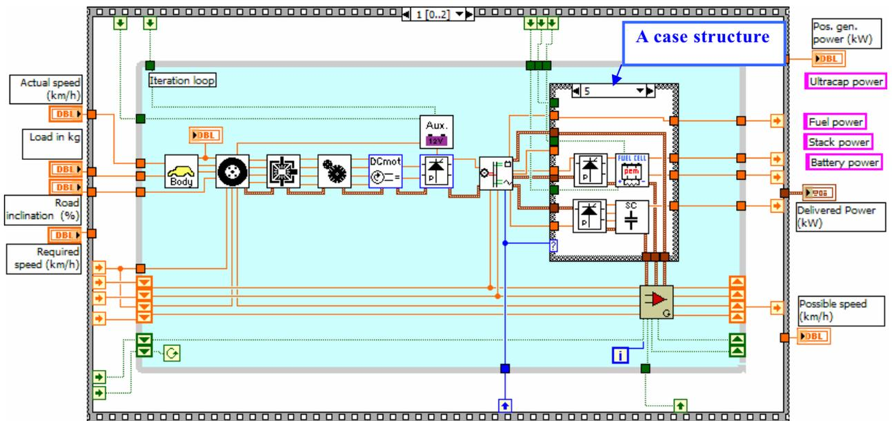
Fig. 2 SHEV drive train model in VSP with two DC/DC converters in this case [3]
