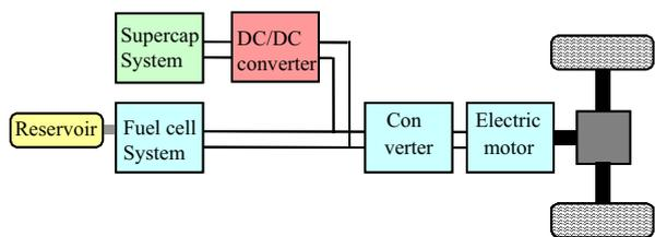
Fig. 8 A series hybrid fuel cell and supercapacitor topology with one DC-DC converter connected to the supercap [4]
