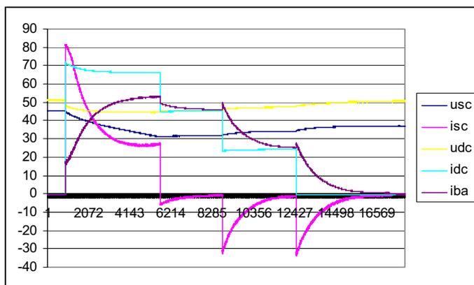
Fig. 11 Waveforms of voltage and current in case only with a DC/DC converter of the supercapacitors (10ms/dot) [7]
