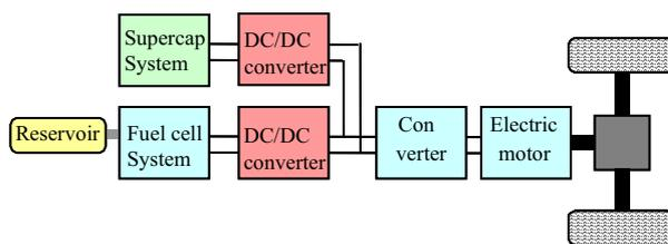
Fig. 5 A series hybrid fuel cell and supercapacitor topology with two DC-DC converters [4]
