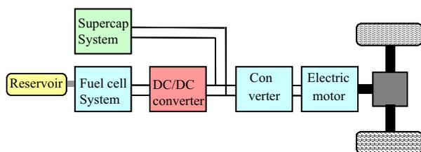
Fig. 7 A series hybrid fuel cell and supercapacitor topology with one DC-DC converter connected to the fuel cell [4]
