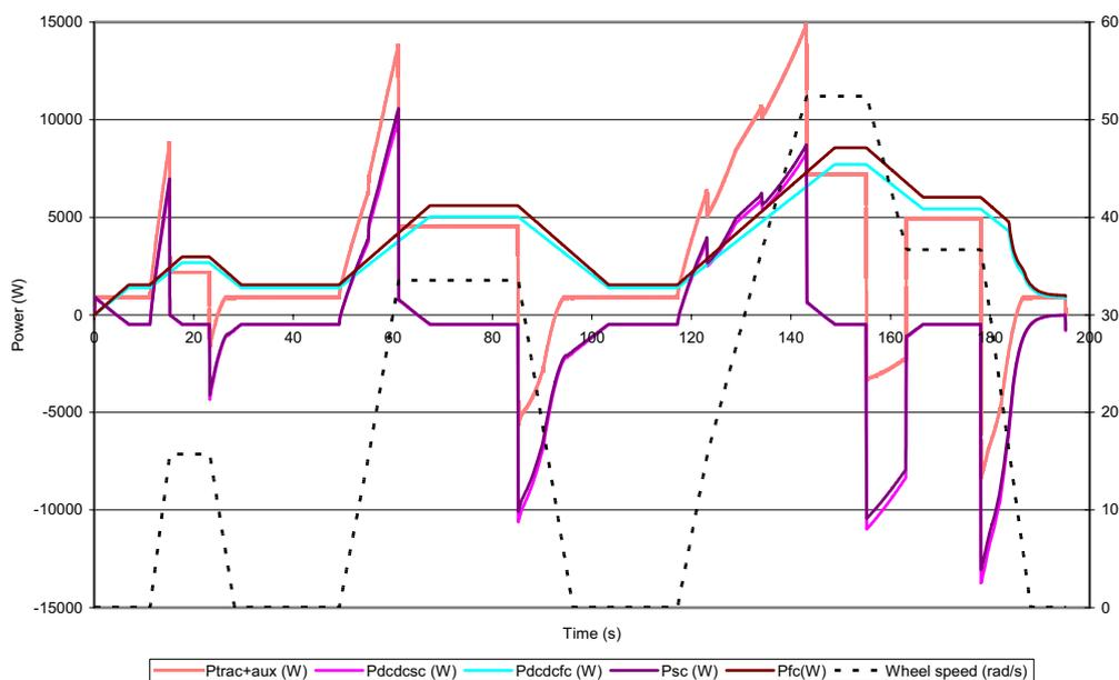
Fig. 3 Power flow in the series hybrid fuel cell and supercapacitor topology with both DC-DC converters [4]
