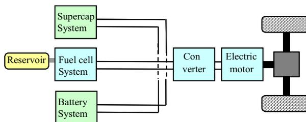
Fig. 6 A series hybrid fuel cell and supercapacitor topology without DC-DC converter [4]
