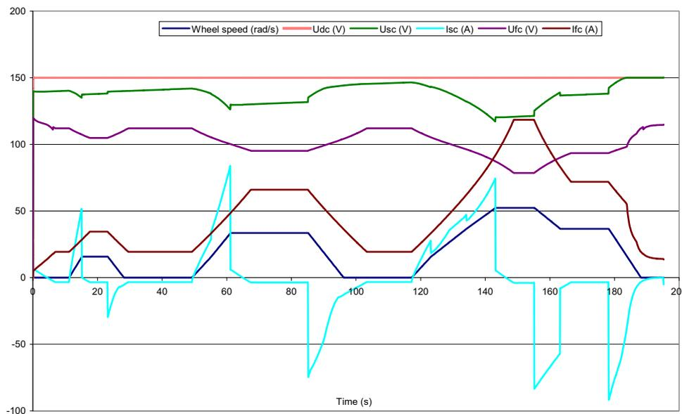
Fig. 4 Currents, voltage and speed of the series hybrid fuel cell and supercapacitor topology with both DC-DC converters [4]
