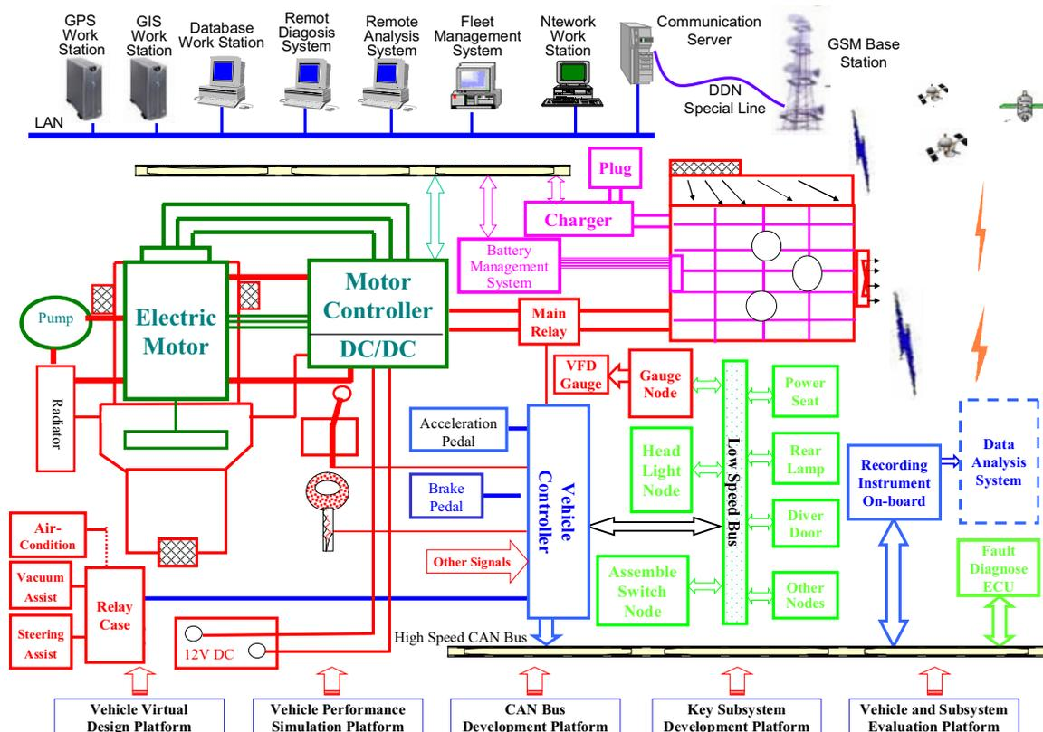
Fig. 1 Technical Configuration of advanced electric vehicle
