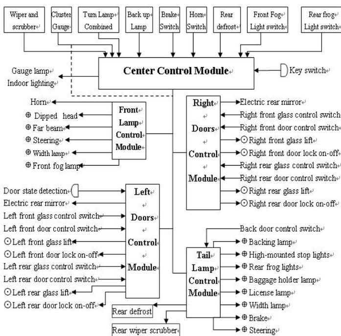
Fig. 4 Network Topology of Body Comfortable System
