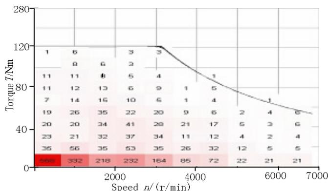
Fig. 7 Distribution of Motor Operation Point
