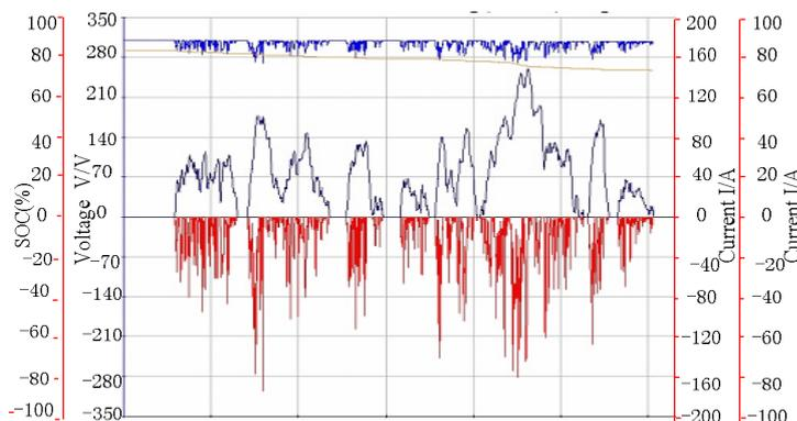
Fig. 6 Running Parameter in Tianjin City Drive Cycle
