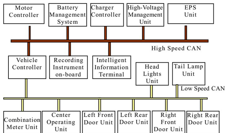
Fig. 3 Vehicle Control System Configuration
