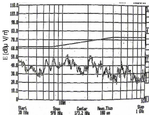
Fig. 9 Plane Polarization Peak Scan Chart
