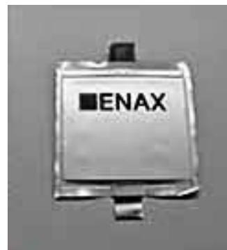
Figure 6: Layered type laminate sheet cell.
