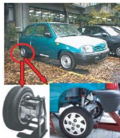
Fig. 1 “UOT March II” and its in-wheel motors
