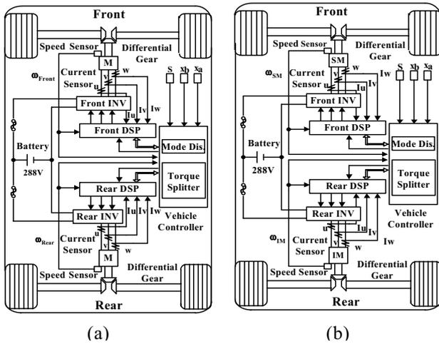
Fig. 1. Structure of EV drive systems. (a) EV with a failsafe structure. (b) Prototype EV that realized the EV with the failsafe structure shown in Fig. (a).
