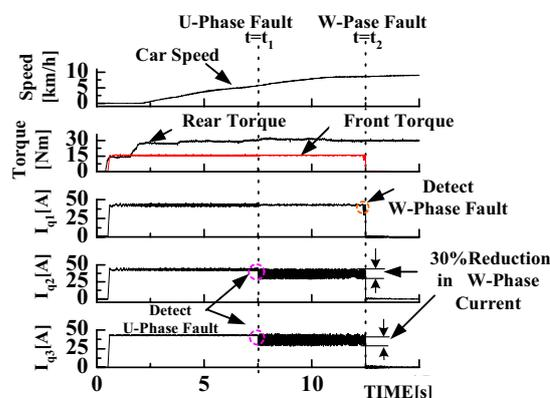
Fig.13. Verification of the proposed failsafe control methods when the current sensors of the front drive system fail in an experiment using the prototype EV.
