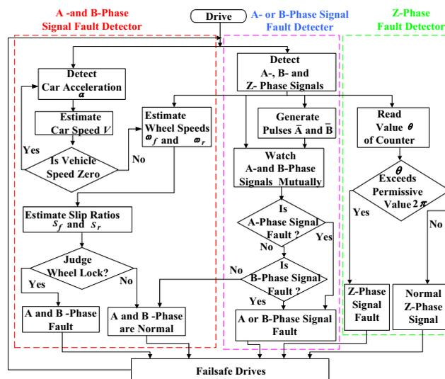
Fig.9. Procedures for performing the failsafe control when the speed sensor failed.
