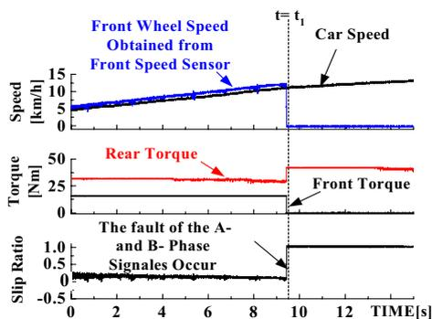
Fig.15. Verification of failsafe control methods when the A- and B-phase signals of the front speed sensor failed.
