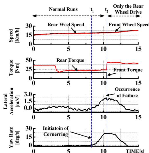
Fig.18. Verification of failsafe control methods when the front wheel drive system fails while cornering.
