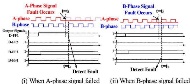
Fig.11. Timing charts for explaining A- or B-phase signal fault detected by circuits shown in Fig.10.
