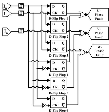
Fig. 5. Structure of circuits to detect the one-phase fault.
