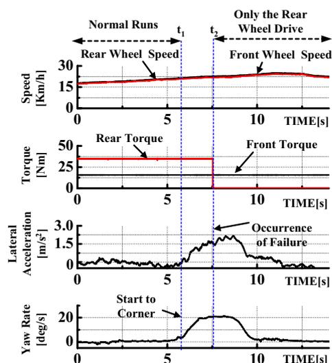
Fig.20. Verification of failsafe control methods when the rear wheel drive system fails while cornering.
