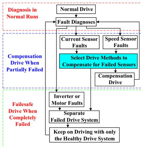
Fig.2. Procedures to execute failsafe control methods suitable for the EV shown in Fig.1.
