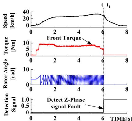
Fig.16. Verification of failsafe control methods when the Z-phase signal of the front speed sensor failed.
