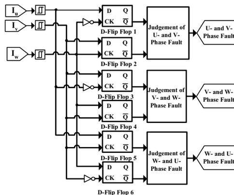
Fig.7. Structure of circuits to detect the two-phase fault.
