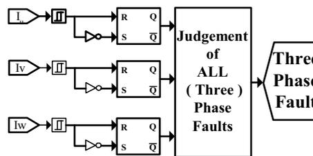
Fig.8. Structure of circuits to detect the three-phase fault.
