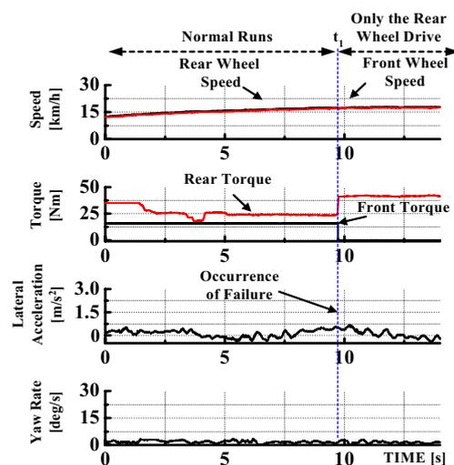
Fig.17. Verification of failsafe control methods when the front wheel drive system fails while going straight.
