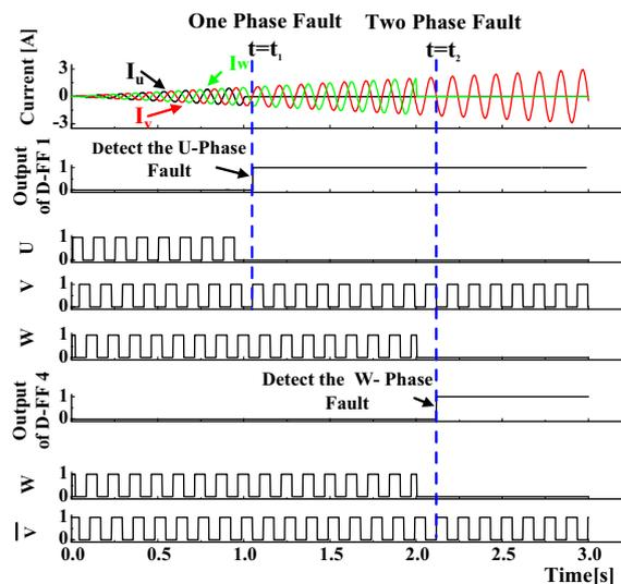
Fig. 6. Simulations for verifying operations of the one- and two-phase fault detection circuits shown in Figs. 5 and 7.
