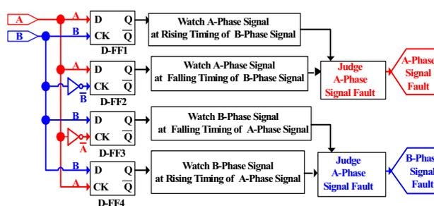
Fig.10. Circuits to detect A- or B- phase signal fault.
