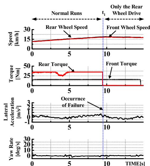
Fig.19. Verification of failsafe control methods when the rear wheel drive system failed while going straight.
