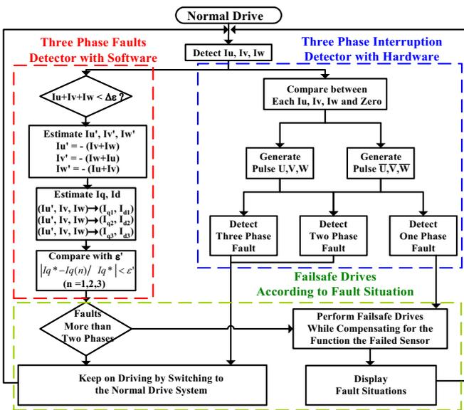
Fig. 4. Failsafe control procedures when current sensors failed.
