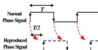
Fig.12. A compensation method when A- or B- phase signal failed.
