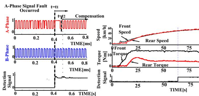
Fig.14. Verification of failsafe control methods when the A-phase signal failed.
