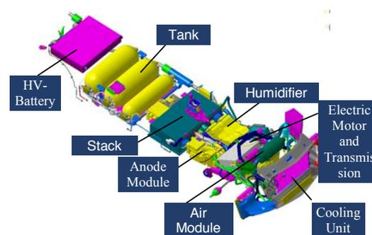
Figure 2: Drive Train B-Class F-CELL
