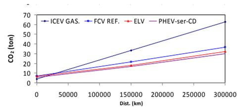
Figure 4: Influence of the distance travelled on full life cycle CO<sub>2</sub> emissions per vehicle.
