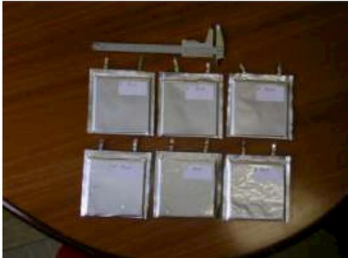
Figure 3: Carbon/IL/carbon symmetric ILHYPOS prototype cells.
