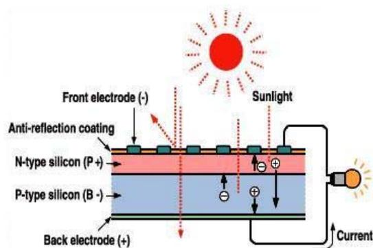
Figure 1: typical schematic diagram of the solar cell
