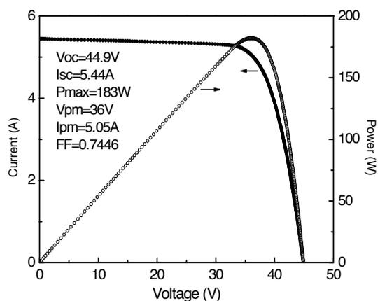
Figure 5: I-V characteristics curves of PV module
