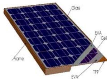
Figure 2: typical schematic diagram of the solar module
