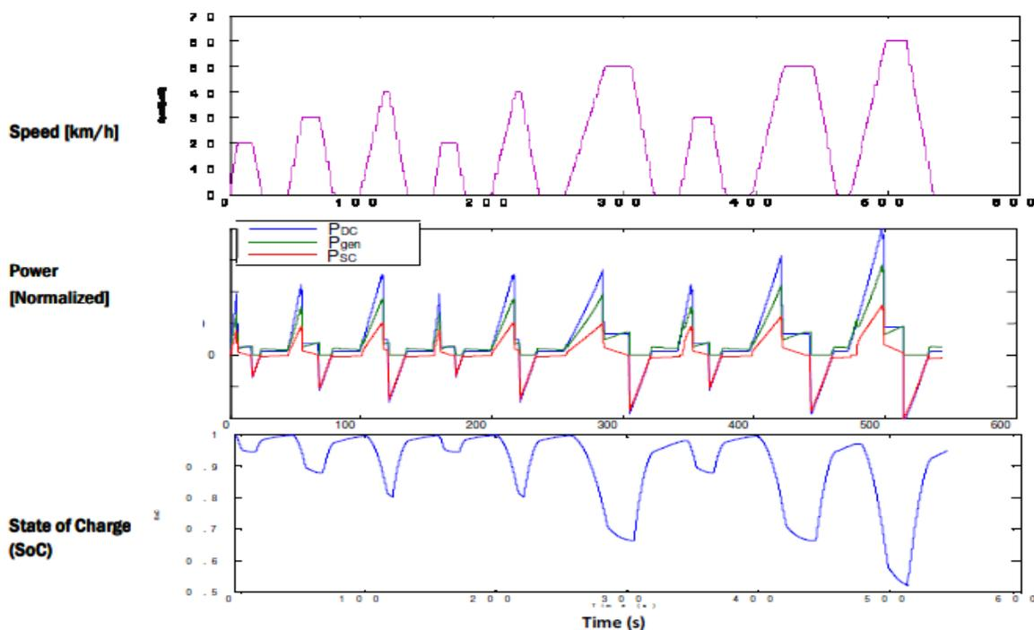
Figure 5a: power flow when kinetic strategy is applied
