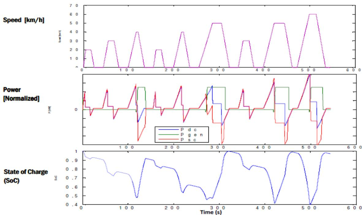
Figure 5b: power flow when ICE on-off strategy is applied
