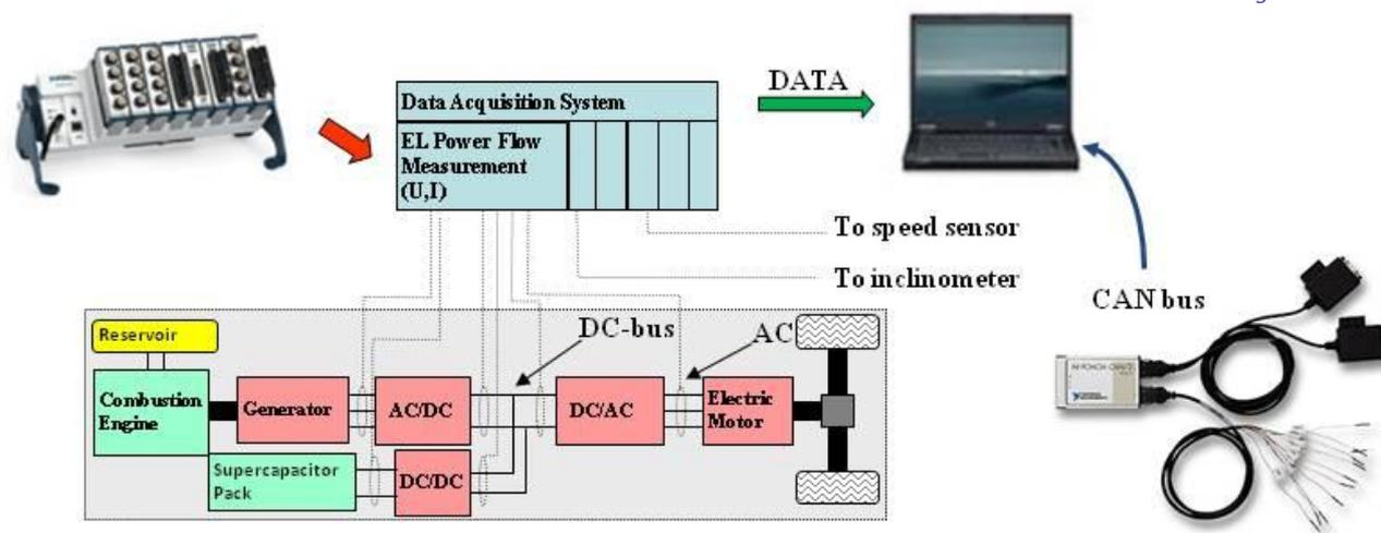
Figure 1: series hybrid structure using supercaps and scheme of the measurement
