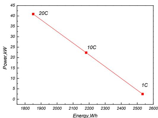
Figure 4: power versus energy of the 288V/8Ah battery system at different discharge rates.
