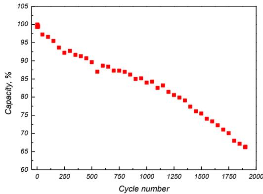
Figure 3: the discharge capacity versus cycle number for the single-cell at room temperature.
