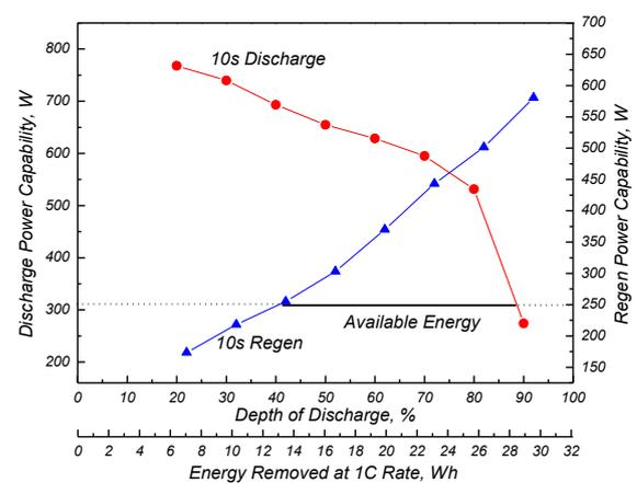
Figure 2: Discharge and regen power versus DOD and Energy removed at 1C rate for the single-cell.
