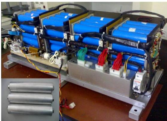
Figure 1: the picture of the 288V/8Ah battery system, the inset represents the single-cells.
