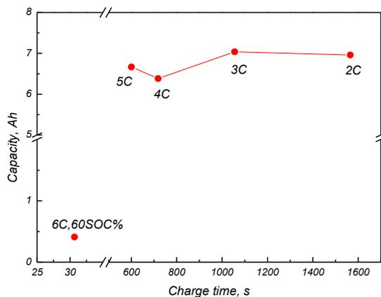
Figure 7: the capacity of constant current charge versus time at different rates.
