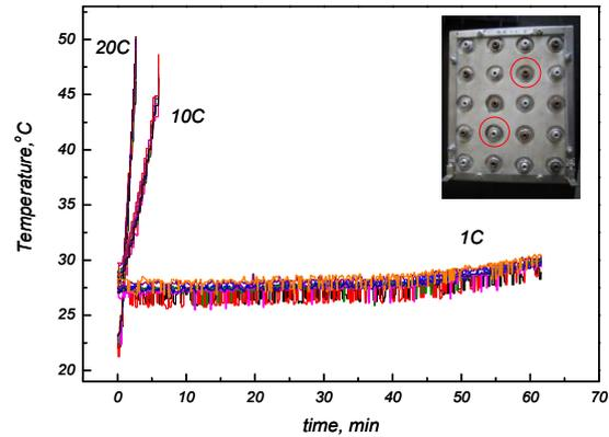
Figure 5: temperature versus time of the 288V/8Ah battery system at different discharge rates, the surface temperature of single-cell marked with red circle is monitored in each module, and the surface temperatures of eight single-cells were detected.
