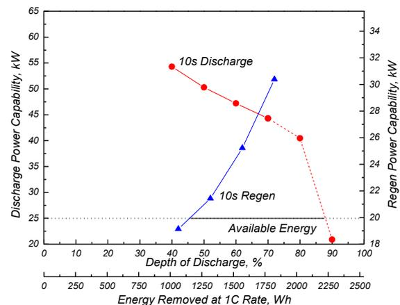
Figure 8: Discharge and regen power versus DOD and energy removed at 1C rate for the battery system. The values of discharge power capability at the 80% and 90% DOD are equal to the values of discharge power capability of single-cell at the 80% and 90% DOD time the average value of the ratios of discharge power capability (battery system and single-cell) at the 40%, 50%, 60% and 70% DOD, respectively.
