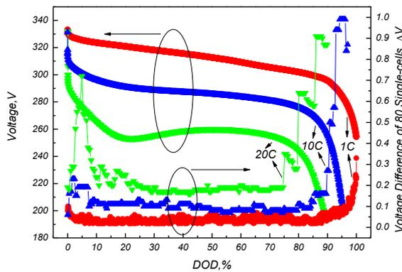
Figure 6: the voltage of battery system versus DOD and the voltage difference of 80 single-cells versus DOD at different discharge rates. The value of voltage difference is equal to the maximum voltage minus the minimum voltage of 80 single-cells in the battery system at the same DOD.
