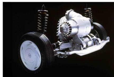
Fig. 4: Volvo ECC's AGT/M-E generator to power the serial HEV's E-M motor [5]
