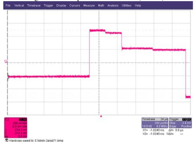
Figure 8: The a-phase stator voltage (4V/div)
