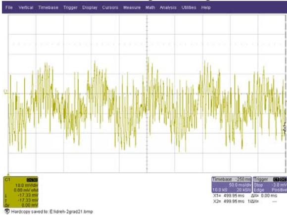
Figure 14: The a-phase stator current (5A/div)
