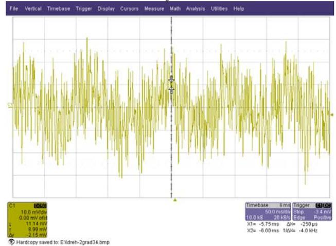
Figure 7: The a-phase stator current (5A/div)
