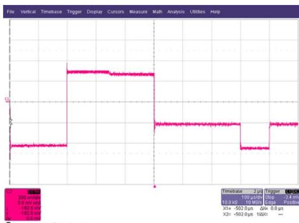
Figure 4: The a-phase stator voltage (4V/div)
