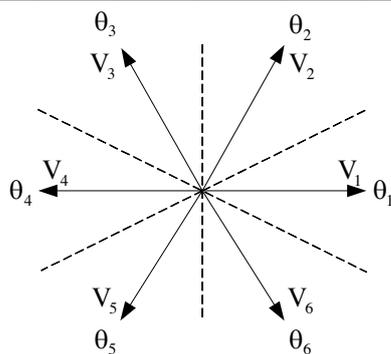
Figure 6: Voltage vectors and stator flux sectors
