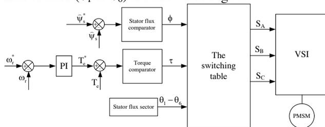
Figure 5: The diagram of PMSM DTC system using switching table
