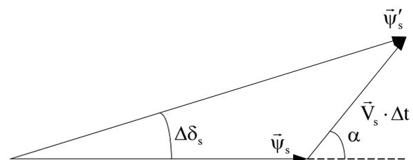
Figure 9: The move of stator flux vector due to the application of voltage vector
