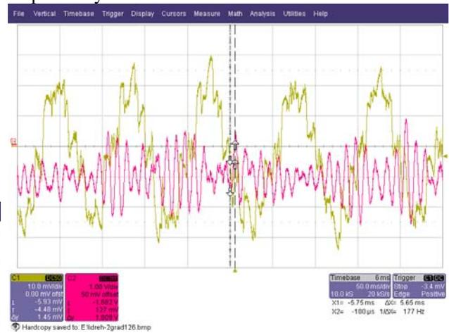
Figure 17: The a-phase stator current (20A/div) and the load torque (10Nm/div)
