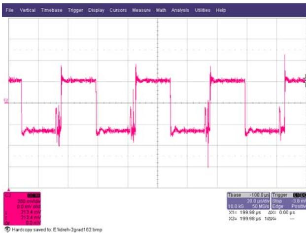
Figure 15: The a-phase stator voltage (4V/div)
