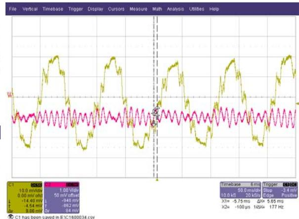
Figure 18: The a-phase stator current (20A/div) and the load torque (10Nm/div)
