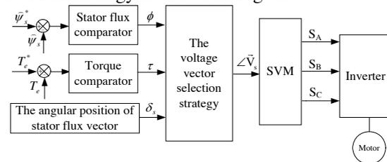
Figure 13: The diagram of the DTC system using voltage vector selection strategy
