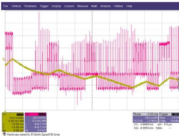
Figure 16: The a-phase stator current (5A/div) and stator voltage (4V/div)
