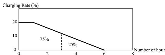
Figure 4: Battery charging characteristics (6-hour charge).
