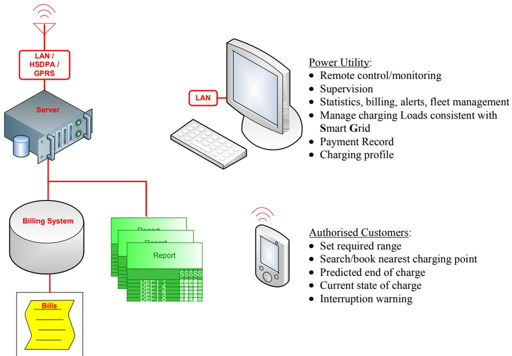
Figure 7: Schematic of the system server, control console and remote access by customers.
