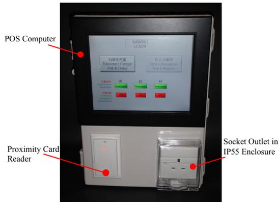
Figure 8: Experimental prototype.
