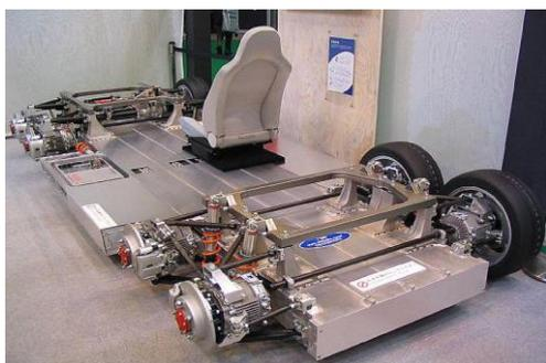
Figure 3: Eliica 8WD Internal structure
