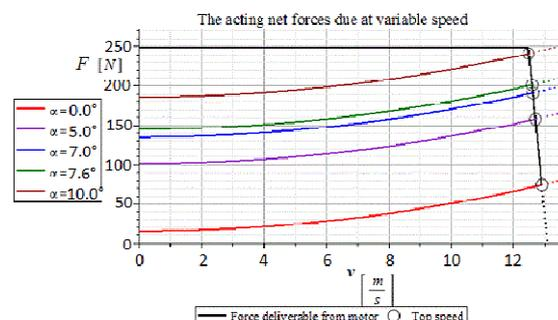
Figure 5: LEM-130-95S motor. FEM's driving characteristics at full throttle and variable hill climbing angle, force over speed.
