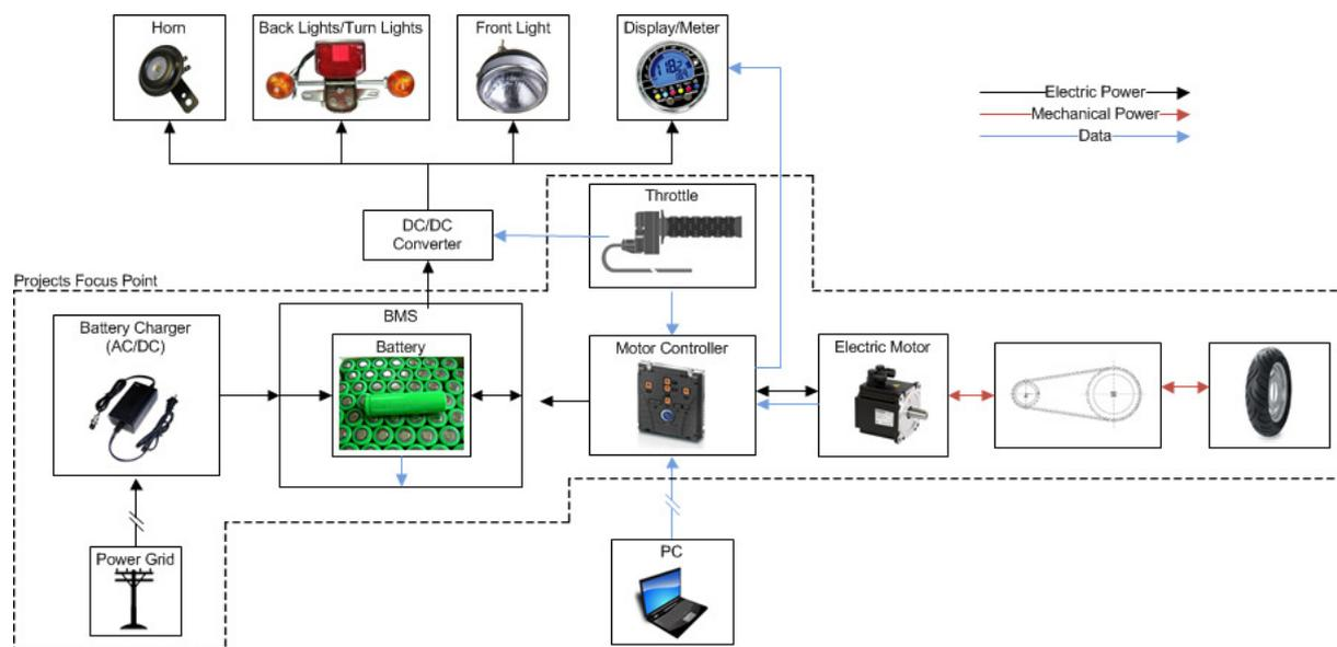
Figure 2: Block diagram of the FEM electrical system
