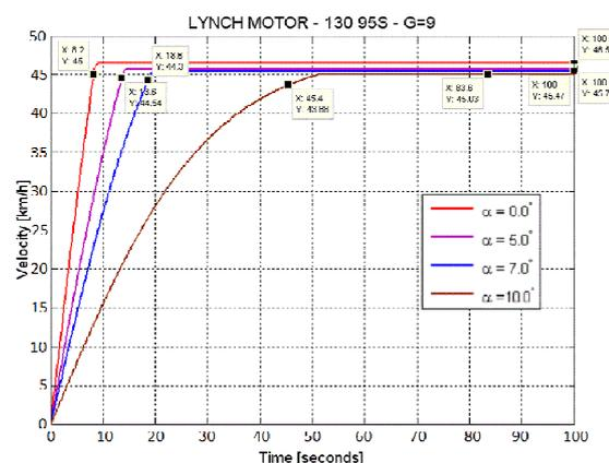
Figure 6: LEM-130-95S motor. FEM's driving characteristics at full throttle and variable hill climbing angle, speed over time.
