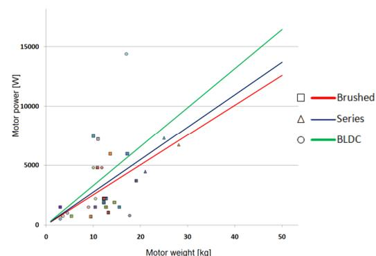
Figure 4: Weight comparison of brushed DC, series and BLDC motors, where the red, blue and green lines represent the average fitted value.
