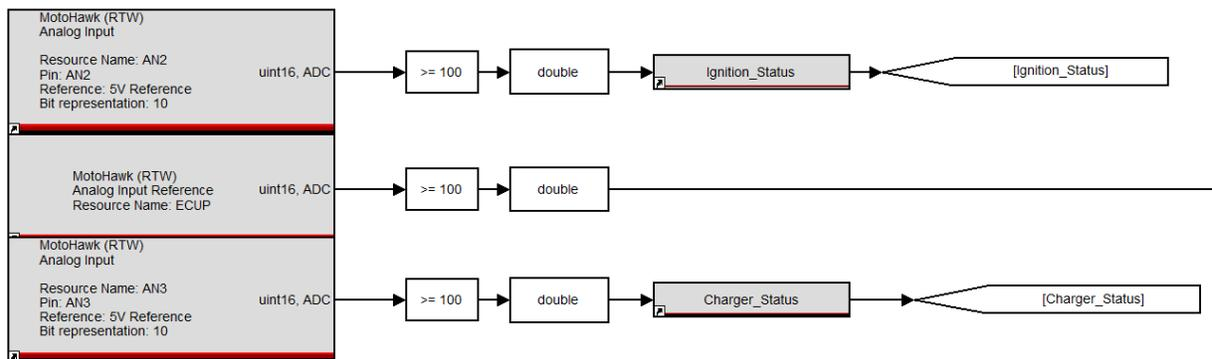
Figure 10 - HIL-Deployment HVSC Input Block Example
