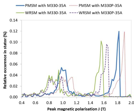
Figure 3: Histograms of  $J_{\text{peak}}$  (= relative occurrence of peak magnetic polarisation evaluated over one electrical period) in the stator for both topologies and both reference materials (M330-35A and M330P-35A). The highest peak corresponds with the polarisation in the stator teeth. For M330-35A this peak is at 1.81T for PMSM and 1.57T for WRSM.
