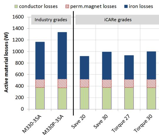
Figure 4: for the PMSM case, active material losses (conductor losses, permanent magnet losses and iron losses) as a function of material choice. Conductor and magnet losses only vary slightly (min. value is only 2% lower than max for conductor losses, and min. value is 9% lower than max for magnet losses).
