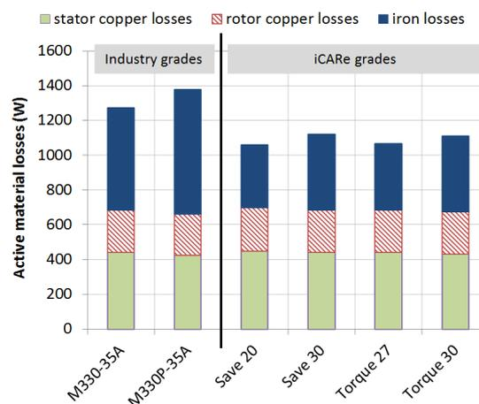
Figure 5: for the WRSM case, active material losses (conductor losses, permanent magnet losses and iron losses) as a function of material choice. Conductor only vary slightly (min. value is only 5% lower than max).
