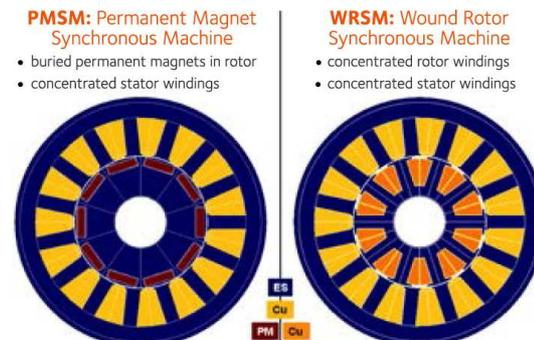
Figure 1: E-machine topologies under study: PMSM (left) and WRSM (right), both having a nominal mechanical power  $P_{\text{nom}} = 31\text{kW}$  at  $f_{\text{nom}} = 400\text{Hz}$ .
