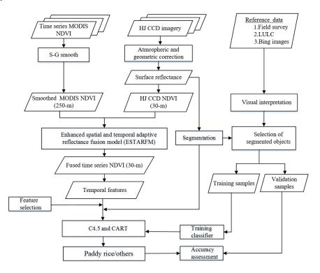
**Figure 3.** Flowchart of fine resolution paddy rice classification combining temporal features from time series coarse resolution data.
