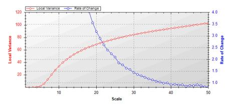
**Figure 6.** Graph of local variance (LV) and rate of change (ROC) at different scales for HJ CCD images with shape: 0.1 and compactness: 0.7.
