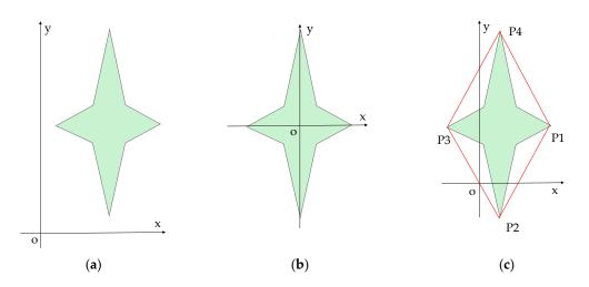
**Figure 4.** Transformation method of center moments and local moments: (**a**) Original position of the polygon, (**b**) moving the origin of coordinates to the centroid of the polygon; and (**c**) the red polyline is the boundary of convex hull, moving the origin of coordinates to the point on the boundary of convex hull.
