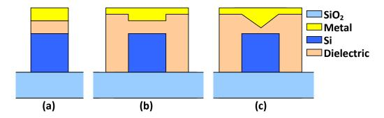
**Figure 5.** Cross sections of silicon hybrid plasmonic waveguides with a standard metal cap [12] (**a**); an inverted metal rib cap [42,43] (**b**); and an inverted metal wedge cap [44,45] (**c**), respectively. [86]
