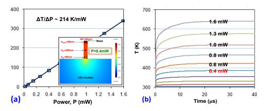
**Figure 11.** (a) The stable temperature variation as the power increases; inset: the simulated temperature profile when a 10  $\mu$ m-long silicon hybrid plasmonic waveguide is heated by an power of 0.4 mW; (b) the temporal response when it is heated with different powers [107].
