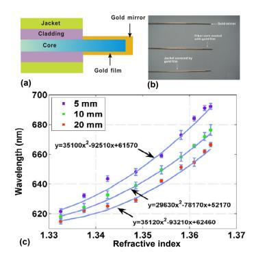
**Figure 13.** (a) Structure of a reflection type SPR fiber optic sensor; (b) Photo of SPR fiber optic sensors; (c) The resonance wavelength shift as the refractive index of the ethanol-water mixture increases in the range from 1.33 to 1.37 [112].
