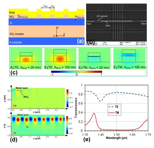
**Figure 10.** (a) Configuration of a TE-pass polarizer with a grating working for TM polarization; (b) SEM picture for the fabricated polarizer; (c) The modal field profiles when the SiO<sub>2</sub>-slot thickness  $h_{SiO2}$  are chosen differently ( $h_{SiO2} = 20$  nm, and 100 nm, respectively); (d) Simulated light propagation in the designed polarizer; (e) Simulated transmission spectral responses for TE- and TM- polarization modes [23].
