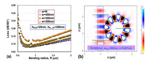
**Figure 3.** (a) The calculated bending loss for bent hybrid plasmonic waveguides (at 1550 nm); (b) The electrical field distribution  $E_y(x, z)$  in a submicron-donut resonator with R = 800 nm, and  $w_g = 80$  nm when it is on-resonance. The other parameters are: the Si core thickness  $h_{Si} = h_{Si_rib} = 300$  nm, the SiO<sub>2</sub> nano-slot thickness  $h_{SiO2} = 20$  nm [16].
