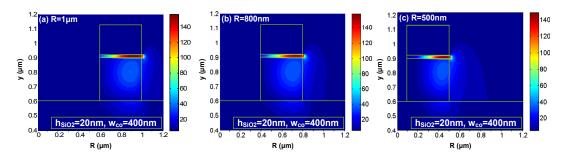
**Figure 2.** Electrical field distribution  $E_y(x, y)$  of the TM fundamental mode for the cases of (a)  $R = 1 \mu m$ ; (b) R = 800 nm; (c) R = 500 nm. The other parameters are: the Si core thickness  $h_{\text{Si}} = h_{\text{Si}} \frac{1}{\text{rib}} = 300 \text{ nm}$ , the SiO<sub>2</sub> nano-slot thickness  $h_{\text{SiO2}} = 20 \text{ nm}$ , the core width  $w_{\text{co}} = 400 \text{ nm}$  [16].
