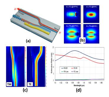
**Figure 7.** (**a**) Configuration of the modified ultrasmall PBS based on an ADC with a silicon hybrid nanoplasmonic waveguide; (**b**) The modal field profiles in a silicon hybrid plasmonic waveguide and an SOI nanowire; (**c**) Light propagation for TM and TM polarizations in the designed PBS; (**d**) The calculated wavelength-dependence of the designed PBS [105].
