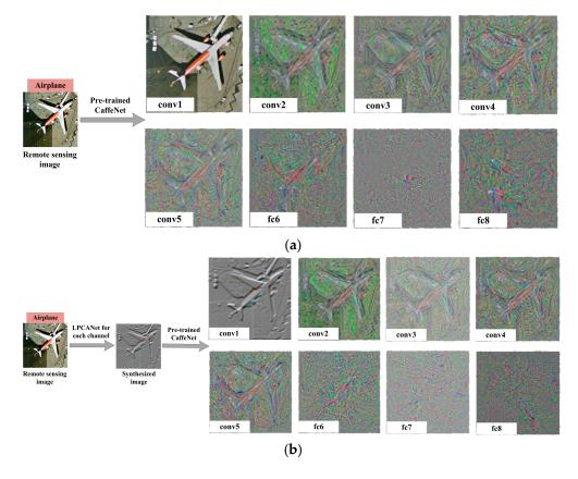
**Figure 12.** Reconstruction of deep CNN activations from different layers of CaffeNet in condition of: (a) Off-the shelf; and (b) Architecture (I). The method presented in [39] is used for visualization.
