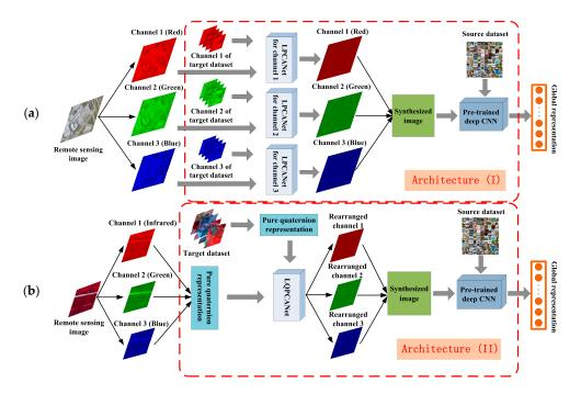
**Figure 7.** Illustration of the two proposed architectures to enhance the generalization power of pre-trained deep CNNs for remote scene classification. In (a) Architecture (I), we use linear PCA networkto synthesize the spatial information of remote sensing imagery in each spectral channel. In (b) Architecture (II), after represent the remote sensing imagery as pure quaternion, we use linear quaternion PCA network to further synthesize the spectral information of them.
