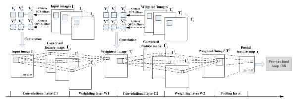
Figure 4. Structure of two-stage linear PCA network (linear quaternion PCA network).
