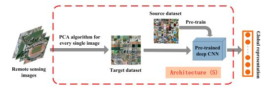
Figure 14. Illustration of the Architecture (S).
