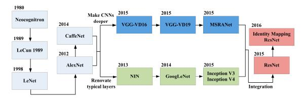
Figure 3. Evolution of the structure of convolutional neural networks.
