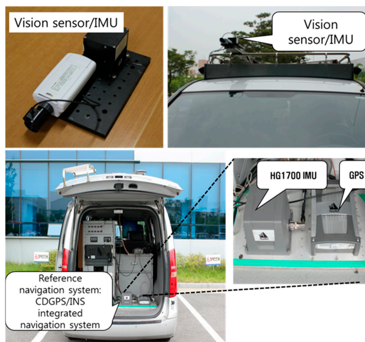
Figure 8. Experimental setup and reference navigation system.
