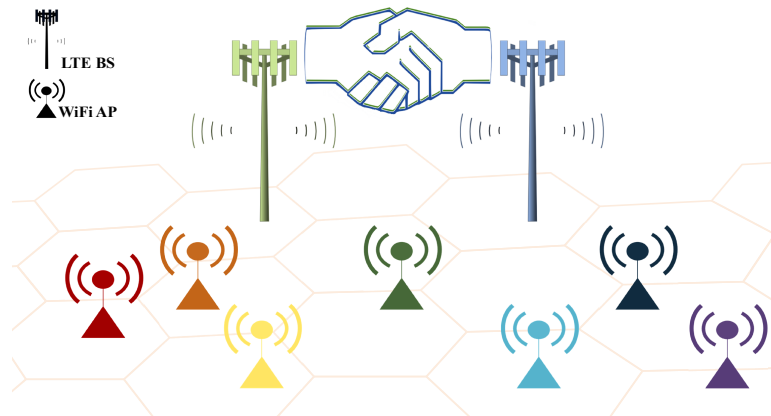
Figure 4. A scenario of collusion between two LTE operators under high density heterogeneous networks in the co-channel of the unlicensed spectrum.
