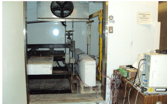
Figure 1. Environmental room including the four point flexural setup, slabs SA and SB.
