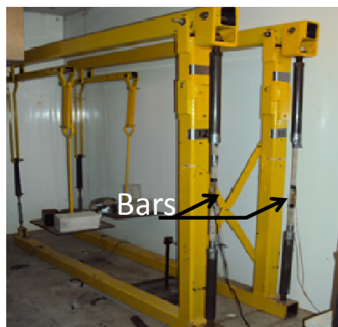
Figure 3. Conditioned tensile test setup of GFRP bars.
