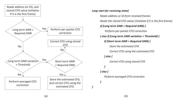
Figure 1. (a) flowchart and (b) algorithm for digital carrier frequency offset (CFO) predistortion.
