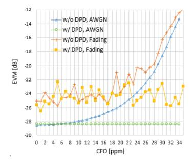
Figure 3. EVM over CFO for channel conditions.
