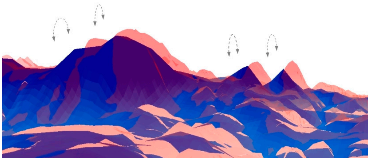
Figure 1. Direct datum-transformation of two different Digital Terrain Model (DTM) databases showing topographic and morphologic inconsistencies, depicted by arrows, which can be resolved only by rigorous local adjustment.
