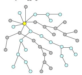
**Figure 7.** Two disjoint aggregation trees rooted at a base station.
