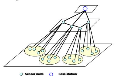
**Figure 5.** Hierarchical wireless sensor network.
