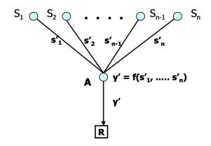
**AH scheme:** The Additively Homomorphic (AH) encryption technique by Castelluccia *et al.* [35] protects privacy against other sensor nodes. The main idea of this approach is to replace the *xor* (Exclusive-OR) operation typically found in stream ciphers with modular addition (+). In the AH scheme, the encryption, decryption and aggregation processes are as given below where c, m, k and M are a cipher-text, a sensor data (message), a key shared with the BS and large integer, respectively.
