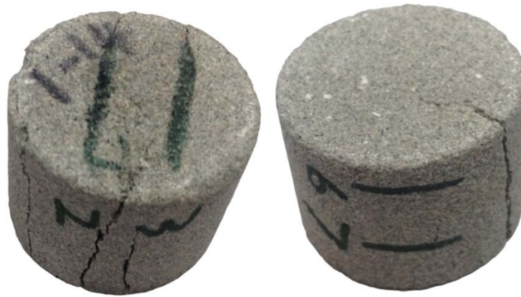
Figure 14. Samples after the impact tests. Even though the sample number for the intermediate strain rate tests is very small, the thin sections for the different directions were obtained from different samples. The thin sections were obtained along the green line.
