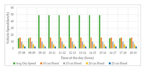
Figure 9. Vehicle speed in relation to floodwater depths.
