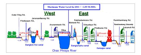
**Figure 4.** Cross-section of Bangkok (Source: Department of Drainage and Sewerage, Bangkok Metropolitan Authority).
