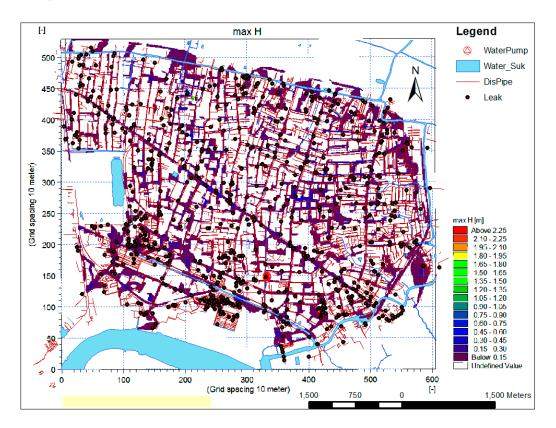
**Figure 14.** Water supply leakage locations overlaid with the 100-year return period flood map; see also [57].
