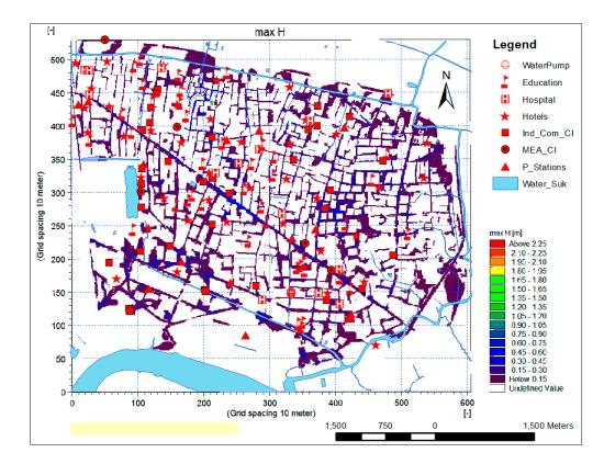
**Figure 11.** Proximity of critical infrastructure in relation to flood prone areas: 1D–2D MIKEFLOOD model result for 100-year rainfall return period (for information concerning local rainfall characteristics, see [56]). MEA, Metropolitan Electricity Authority. (Ind\_Com\_CI stands for *Industries and Commercial Critical Infrastructures* and P\_Stations stands for *Petrol Stations*).
