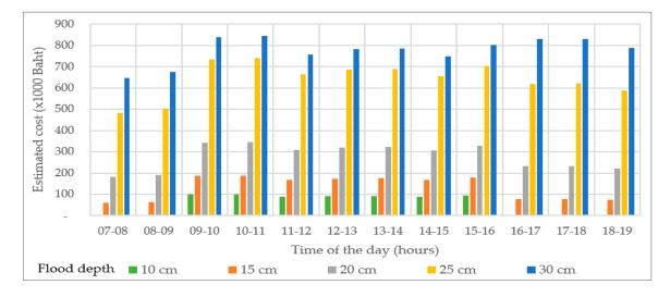
Figure 12. Quantification of impacts: cost of delay time vs. flood depth for Soi Sukhumvit 71.
