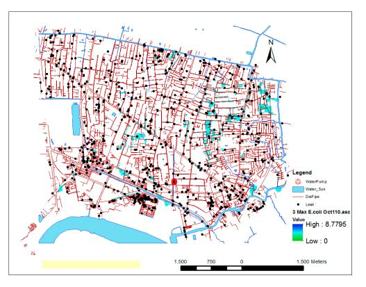
**Figure 15.** Pipe leakage locations in relation to *E. coli* concentrations in floodwaters [42]. Concentrations were obtained from coupled 1D/2D model simulations.
