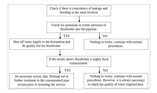
Figure 16. The possible actions to mitigate floodwater intrusion into the water supply system.
