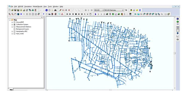
Figure 5. 1D pipe network model coupled with the 2D surface model in MIKEFLOOD.
