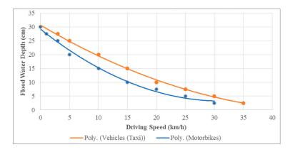
Figure 8. Relationships between floodwater depth and vehicle speed based on interview data.
