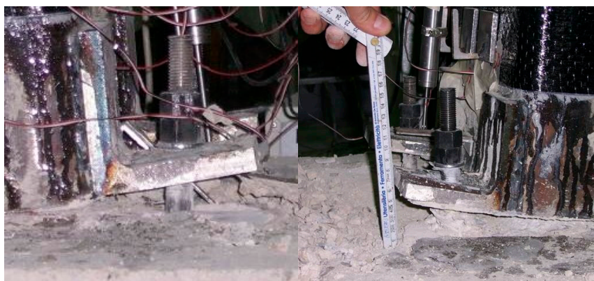
Figure 10. Pull-out of the steel connector from the concrete foundation.
