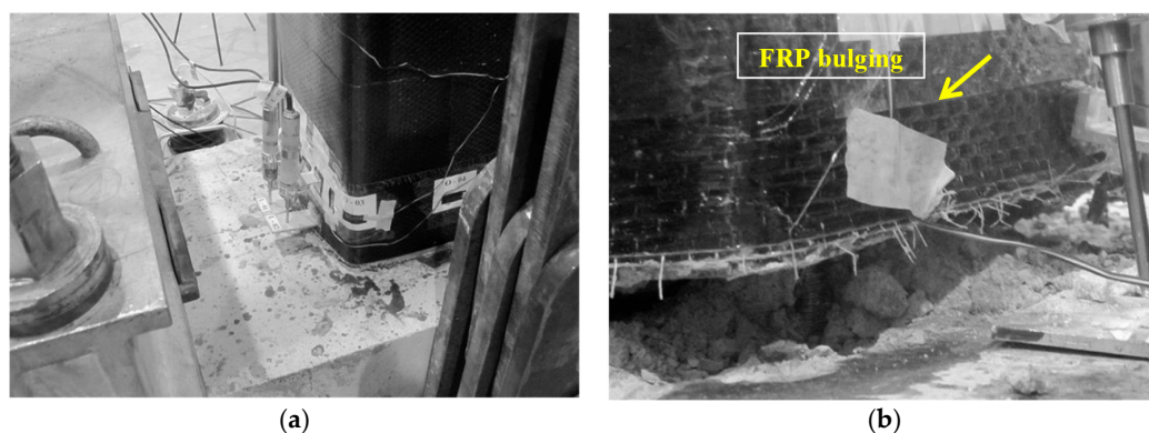
Figure 16. Damage of specimens strengthened with the system “type B”.
