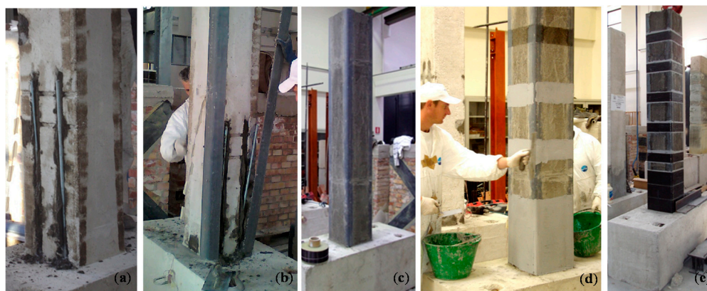
Figure 4. Strengthening procedure: layout "type B".
