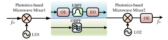
Figure 3. Schematic diagram of photonic an IRM based on multiple-stage frequency conversion.
