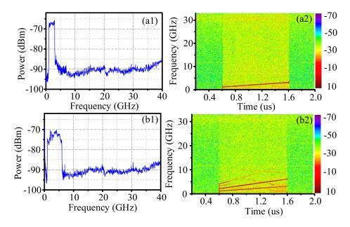
**Figure 8.** (**a1**,**b1**) Electrical spectra and (**a2**,**b2**) time-frequency diagrams of the downconverted results for schemes in (**a1**,**a2**) [30] and (**a1**,**b1**) [25] when an RF signal with 2-GHz bandwidth and corresponding image are received simultaneously.
