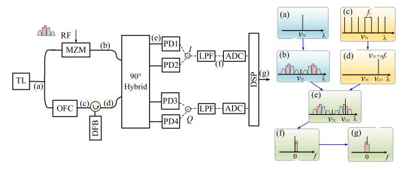
**Figure 9.** Scheme of a photonics-assisted electronic warfare scanning receiver using a photonics-based microwave mixer incorporating a 90° optical hybrid [34].
