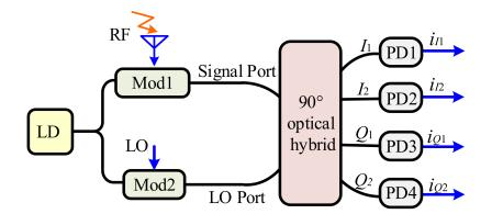
Figure 7. Schematic diagram of a typical photonic IRM using a 90° optical hybrid [25].
