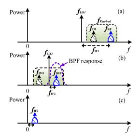
**Figure 4.** Principle of a photonic IRM based on multiple-stage frequency conversion: (**a**) the received RF signal and the location of LO1; (**b**) the downconverted signal using LO1 and the image to be rejected by the bandpass filter (BPF); (**c**) the signal downconverted to the desired output intermediate frequency (IF) band using LO2.
