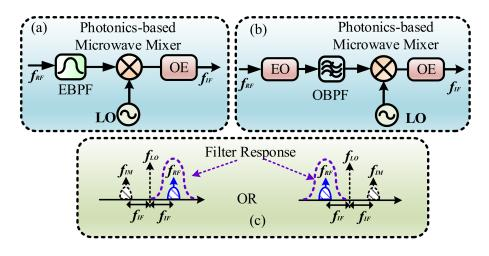
**Figure 2.** Schematic diagram of photonic image-reject mixers (IRMs) based on direct pre-filtering in an (**a**) electrical and (**b**) optical domain; (**c**) pre-filtering principle of IRMs. EBPF: electrical bandpass filter; OBPF: optical bandpass filter; EO: electrical to optical conversion; OE: optical to electrical conversion.
