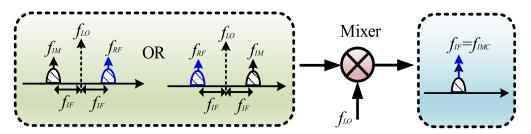
Figure 1. Schematic diagram illustrating image interference.
