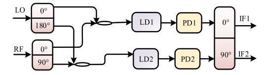
**Figure 6.** A photonic IRM using an electrical 90° hybrid to generate quadrature RFs. LD: laser diode; PD: photodetector [19].
