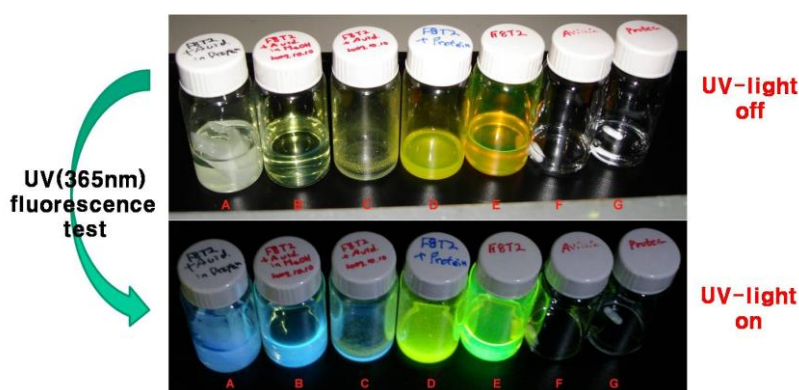
Figure 6. UV (365 nm) fluorescence test with BSA- or avidin-treated biotinylated F8T2. (A) biotinylated F8T2 with Avidin in dioxane. (B,C) biotinylated F8T2 with Avidin in MeOH. (D) biotinylated F8T2 with BSA in MeOH. (E) biotinylated F8T2 in p -Xylene. (F) Avidin in water. (G) BSA in water (up: UV light off; down: UV light on).
