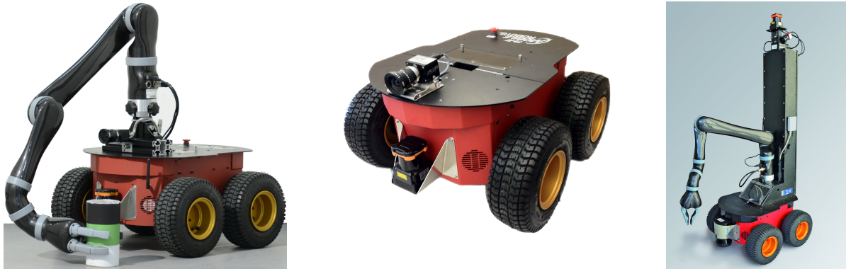
Figure 1. The three types of robots used in Integrated Mission Planning for Distributed Robot Systems (IMPERA). (Left) The mobile robot Stummel with a manipulator arm, 2D LiDAR and color camera. (Middle) The Scout robot equipped with 2D LiDAR and color camera. (Right) The mobile robot Amparo with a manipulator arm and 3D perception unit.
