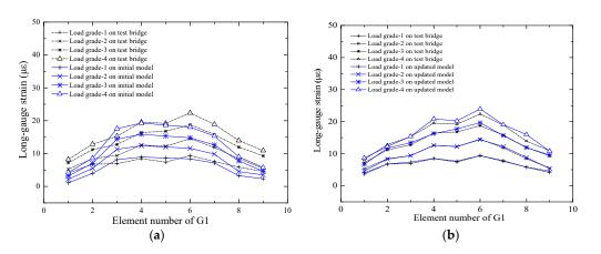
**Figure 15.** Comparison of macro-strains of the G1: (**a**) Comparison between the initial strain and the actual strain; (**b**) Comparison between the updated strain and the actual strain.
