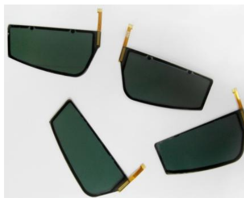
Figure 5. Examples of the fabricated flexible liquid crystal lens.
