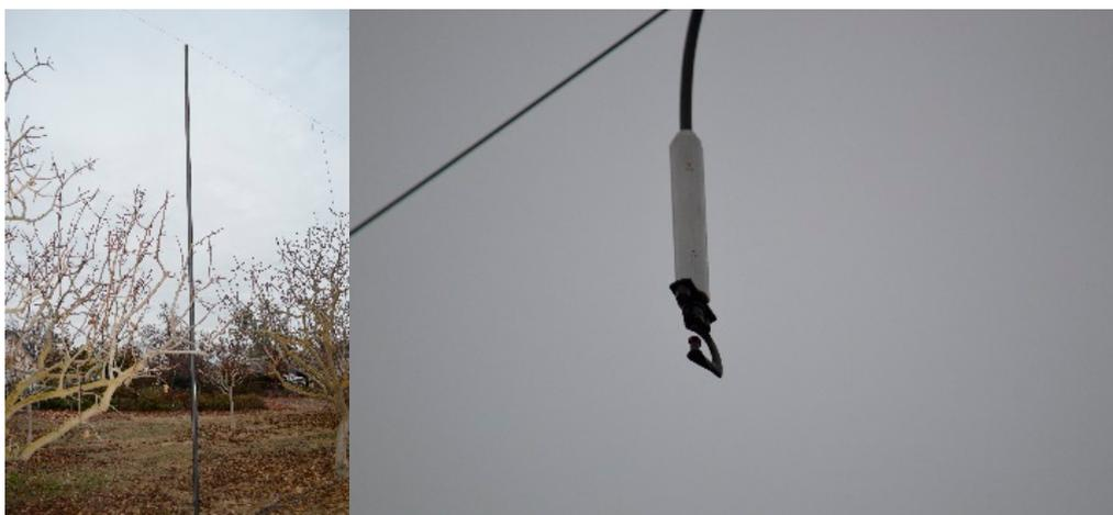
**Figure 3.** Highwire nozzle arrangement above canopy.
