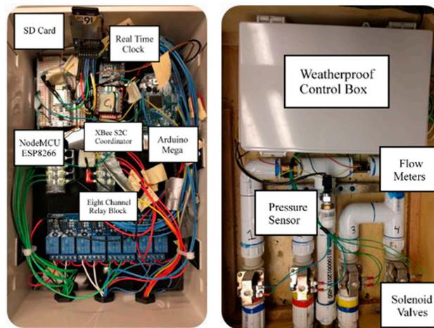
**Figure 9.** The Smart Control (SC) System includes an Arduino Mega 2560 microcontroller, a node MCU Wifi module, a XBee S2C, a real-time clock, eight-channel relay block, solenoid valves, flow meters, and pressure sensor.
