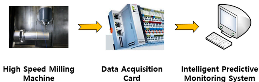
Figure 3. Tool conditions monitoring in high speed milling process.
