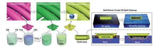
**Figure 11.** Schematic illustration of the fabrication of a superhydrophobic fabric with micronanostructures via a novel mussel-inspired approach and a superhydrophobic cloth boat made from the fabric for self-driven oil spill cleanup. (Reprinted from Reference [130] with permission).
