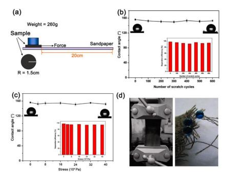
**Figure 8.** (a) Schematic illustration of the methodology of the abrasion test. The variation of water contact angles of the coated fabric (b) scratched by the sandpaper, and (c) stretched by axial tensile forces. Insets are the corresponding separation efficiencies for the oil-water mixture; (d) Images of the stretched textile (left) and water droplets on the broken yarns (right). (Reprinted from Reference [99] with permission).
