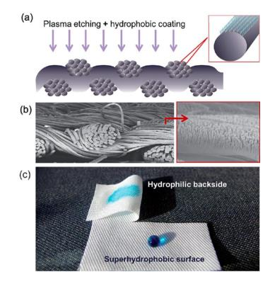
**Figure 9.** Nanostructured fabric surface: (**a**) schematic of plasma-processed fabric surface; (**b**) FE-SEM images of lyocell fabric that was oxygen etched for 20 min; (**c**) Photographic image demonstrating the asymmetric wetting behavior of the plasma-processed lyocell fabric. (Reprinted from Reference [107] with permission).
