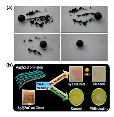
**Figure 14.** (a) Self-cleaning process on a superhydrophobic TiO<sub>2</sub> surface (Reprinted from Reference [148] with permission); (b) Ag@ZnO nanostructured self-cleaning flexible materials with photocatalysis and anti-bacterial activities (Reprinted from Reference [150] with permission).
