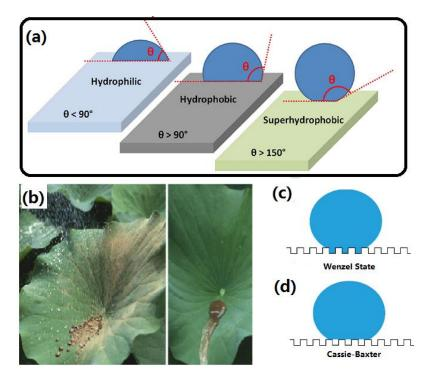
**Figure 1.** (a) The schematic illustration of wetting states of surfaces with different contact angles (Reprinted from Reference [5] with permission); (b) Lotus leaf with typical self-cleaning effect; (c) Wenzel wetting state; (d) Cassie-Baxter wetting state.
