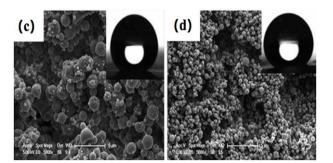
**Figure 6.** SEM images of various polyimide-siloxane mats through the electro-spinning of different poly(amic acid) precursor solutions synthesized by the condensation reaction of 3,3',4,4'-benzophenone tetracarboxylic dianhydride (as a dianhydride) with a mixture of 4,4'-oxydianiline and aminopropyl terminated polydimethylsiloxane (as diamines). (a): PIS-1, (b): PIS-2, (c): PIS-3 and (d): PIS-4 at  $5000 \times$  magnification. (Reprinted from R eference [81] with permission).
