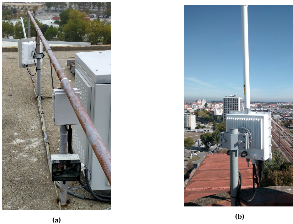
Figure 7. LoRa gateway deployment (a) LoRa gateway deployed in the University of Aveiro; (b) LoRa gateway deployed in Aveiro's Cultural and Congress Center.
