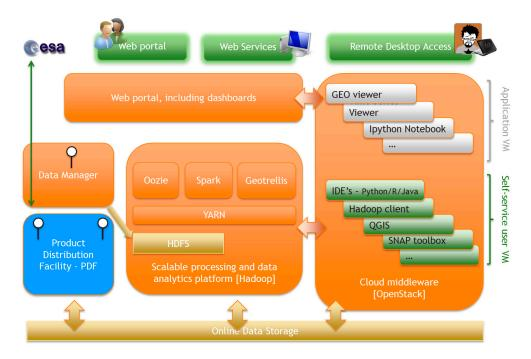
Figure 1. High level architecture diagram of the PROBA-V MEP.
