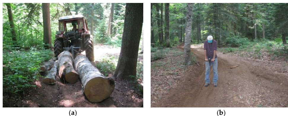
Figure 1. (a) Log skidding on the skid trails; (b) Soil compaction measurement with hand penetrometer on the skid trails.
