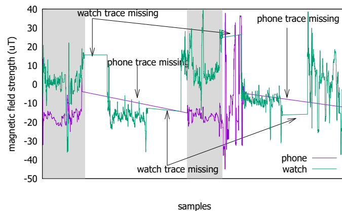
Figure 5. Magnetometer traces from the two mobile devices partially overlap over certain time periods in the Pisa traces.
