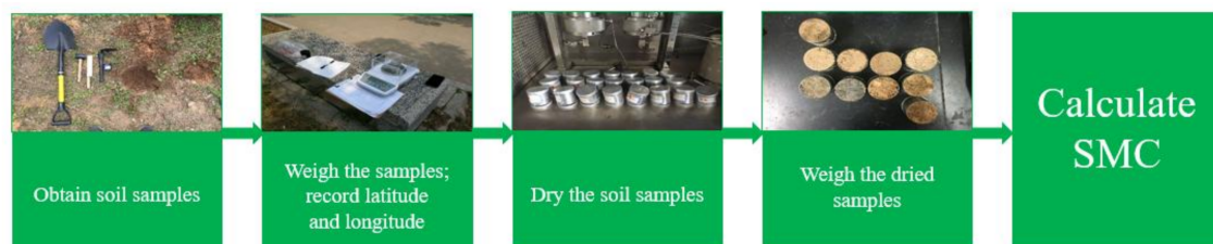
Figure 2. The experimental procedures for obtaining soil samples and calculating the soil moisture content (SMC).
